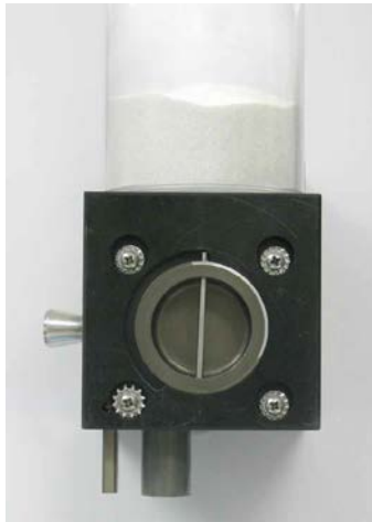
Figure 1: Salt dispenser equipped with gravity fed hopper
